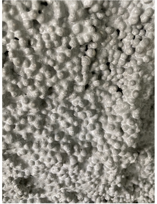
Lightherm beads encapsulated
