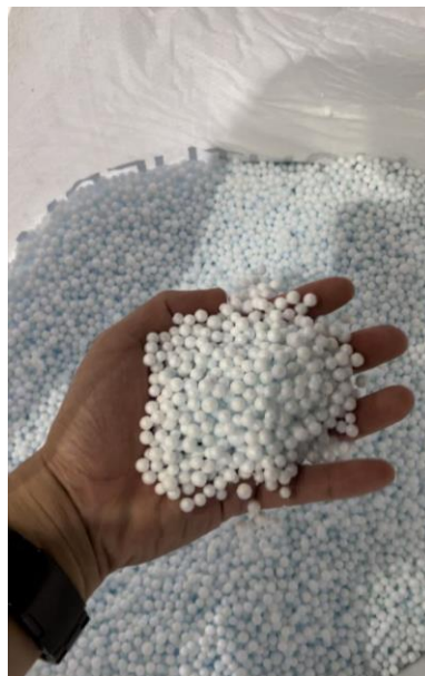
Picture above shown the polyfoam beads blend well with cement without segregation
