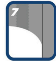
Embed Fireglass Tape Apply thin layer of Skim Coat Base / Render
