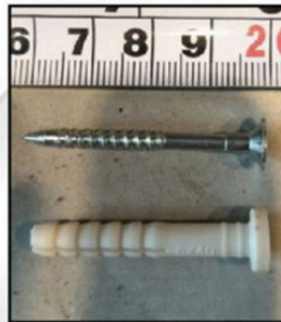
Figure 1: M6 40 Nylon wall plug and screw
