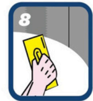
Skim Coat / Render Embed Fibreglass Tape & Top Up with Skim Coat Base / Render
