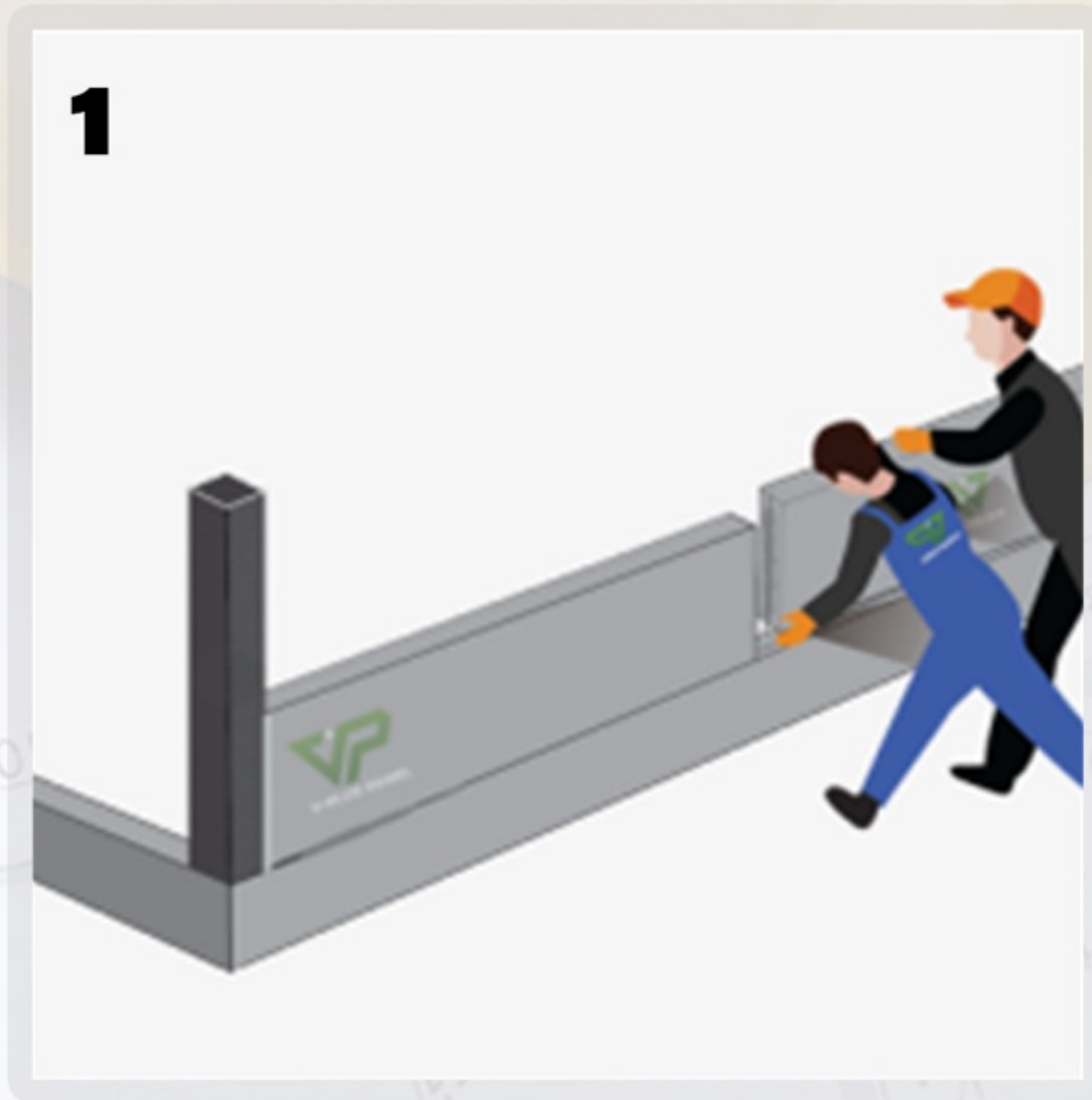
1 Install V-PLUS Panel horizontally attach to column.
