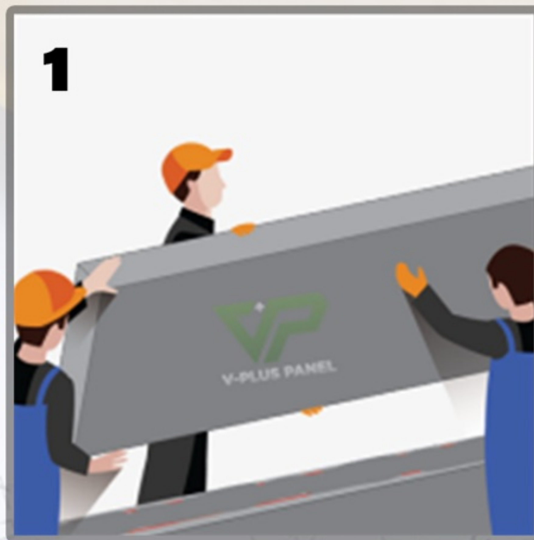
1 Install V-PLUS Panel horizontally attach to column.
