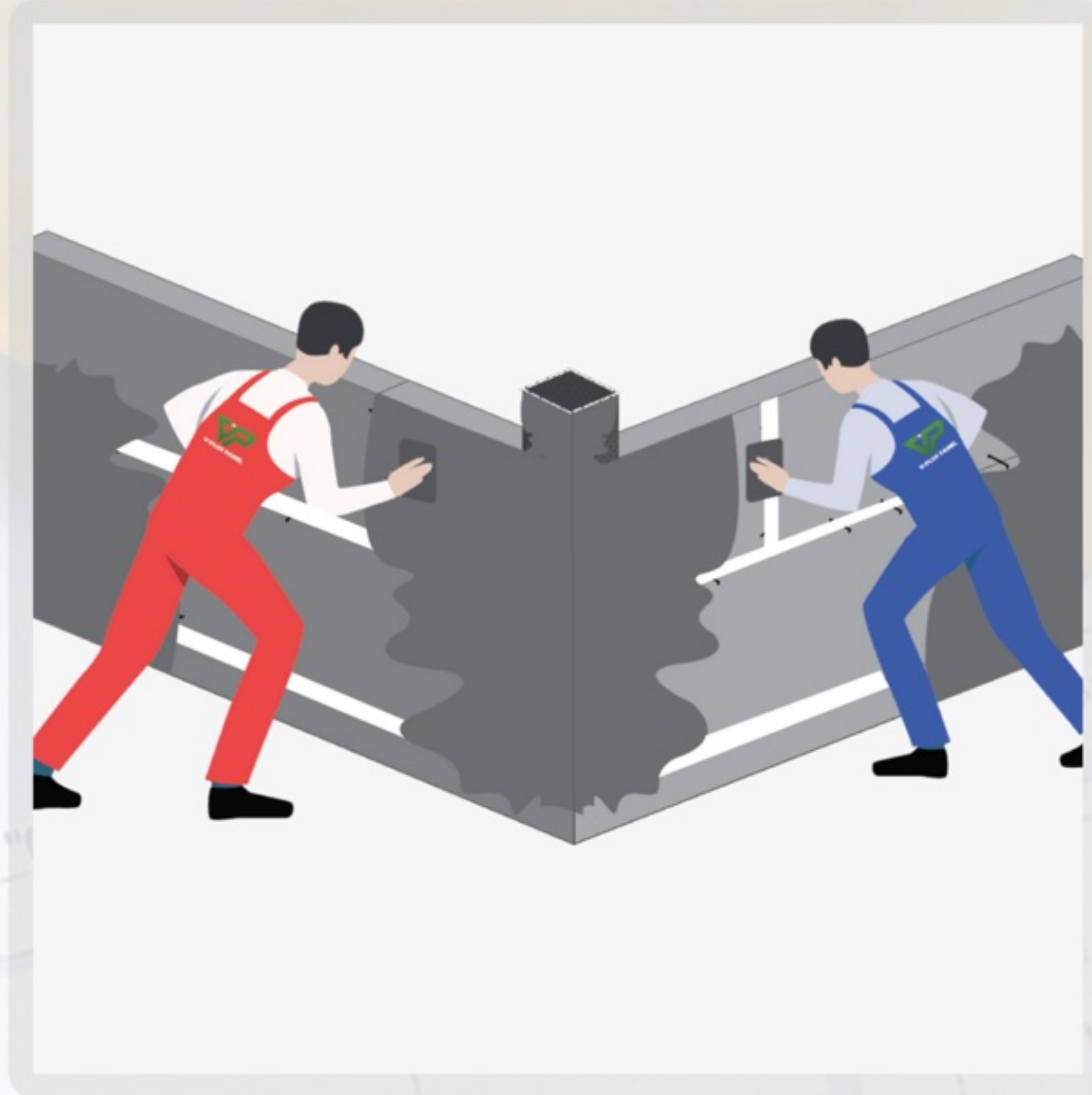
Install fibre Mesh at every jointing.
