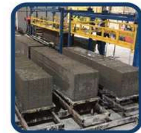
vPanel - Block ( ALC Block - Aerated Lightweight Concrete Block ).
