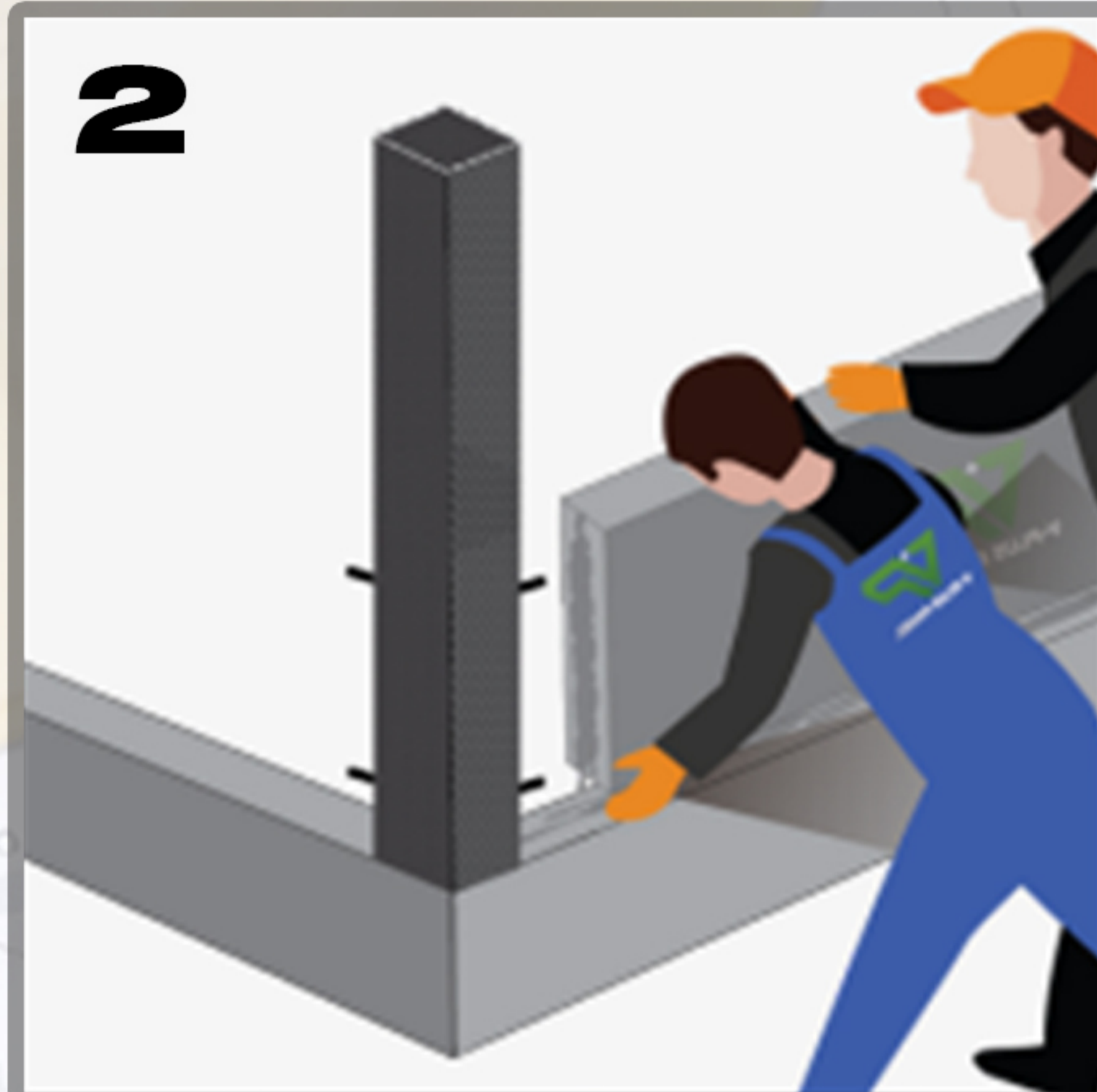
2 before column jointing, Install 6 inches Y10 steel rebar into the column (3 inches in & 3 inches out).
