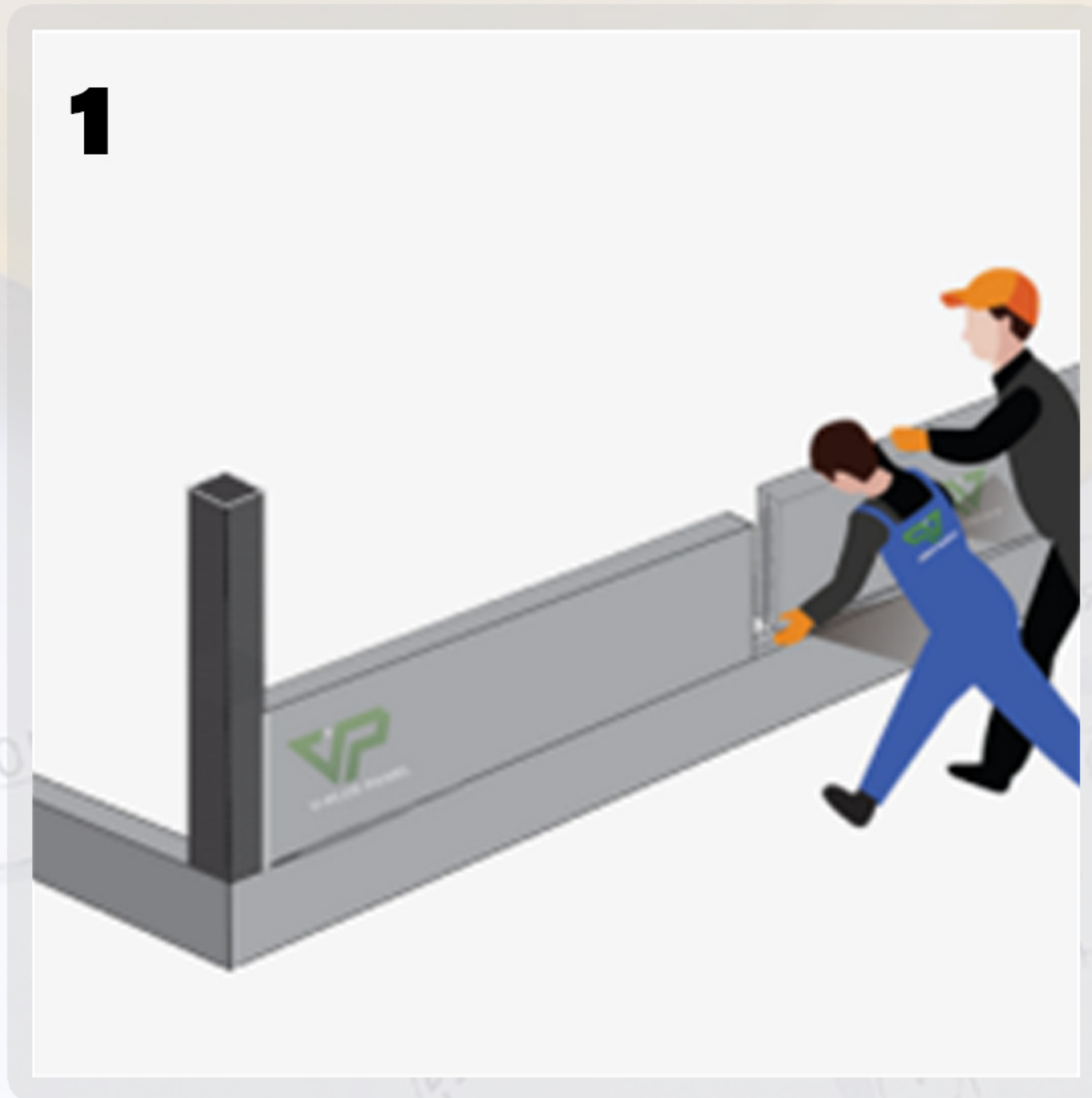
1 Install V-PLUS Panel horizontally attach to column.
