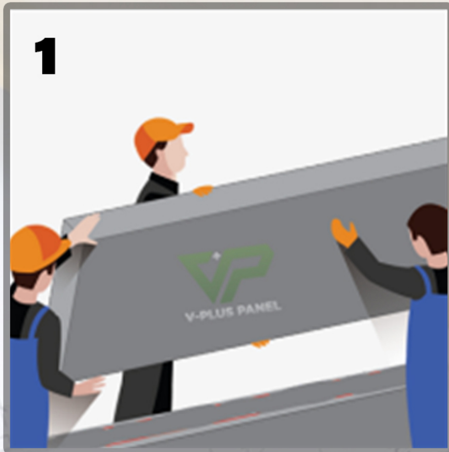
1 Install V-PLUS Panel horizontally attach to column.
