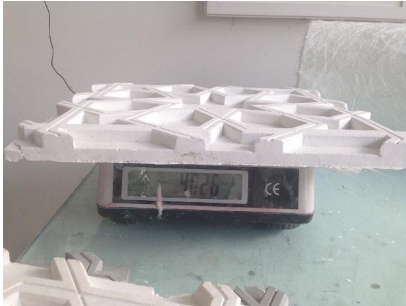
4.026kg, weight before mixing with Politerm Blu
