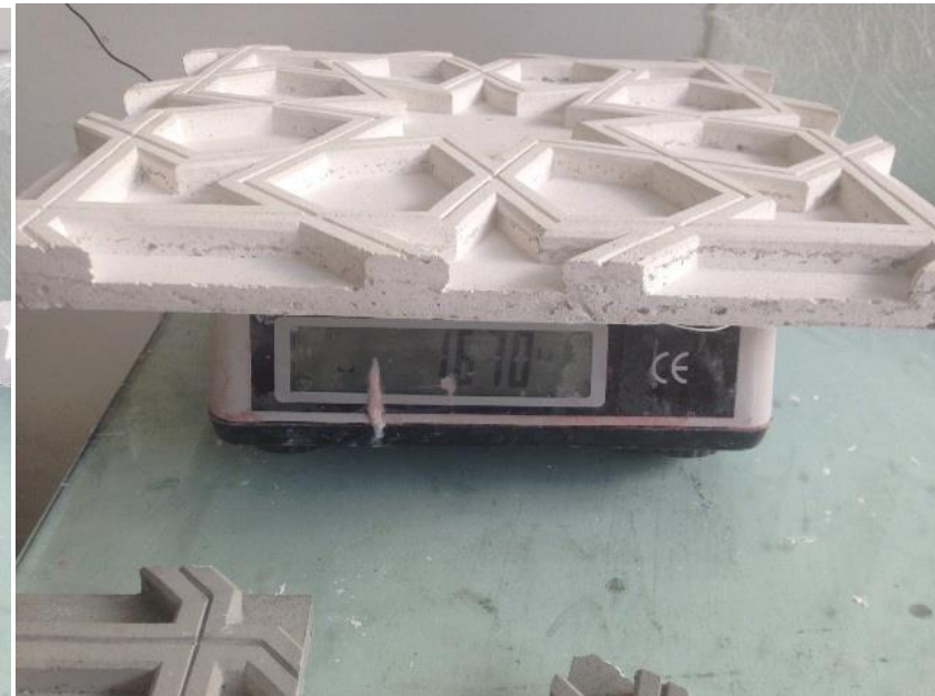
1.670kg ,weight after mixing with Politerm Blu
