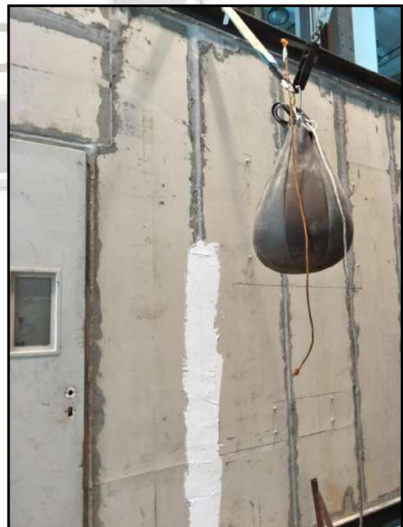
Figure 20: Large softbody impact test
