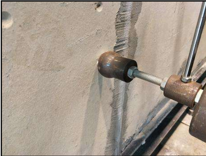
Figure17: : Small hardbody impact test
